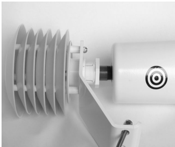
2. Start nut and Insert grey nipple.
